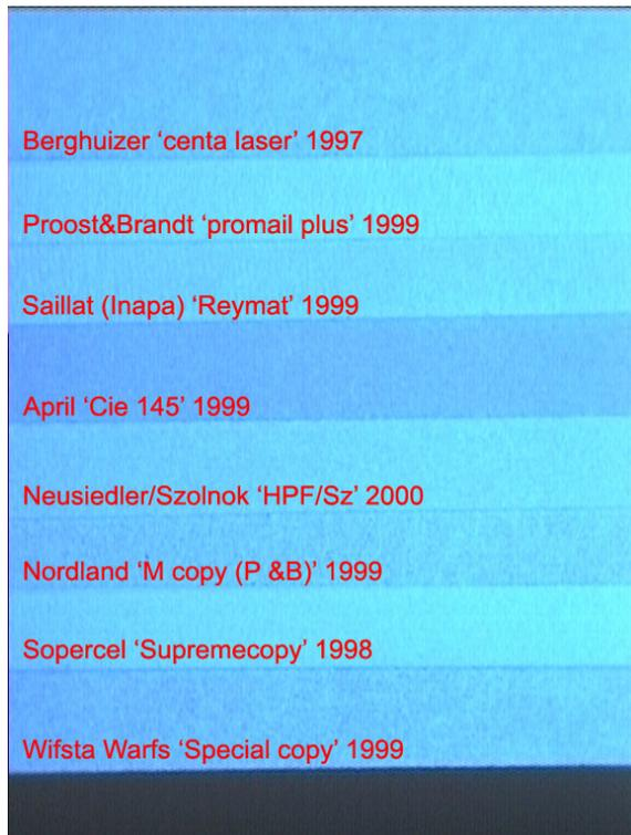
**Figure 11: UV absorption of different modern office papers.**
